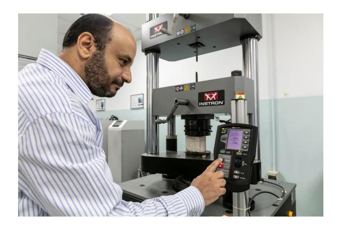
DX600 Static Hydraulic Universal TestingSystems are available in a variety of capacities.They have been developed for high-capacity
