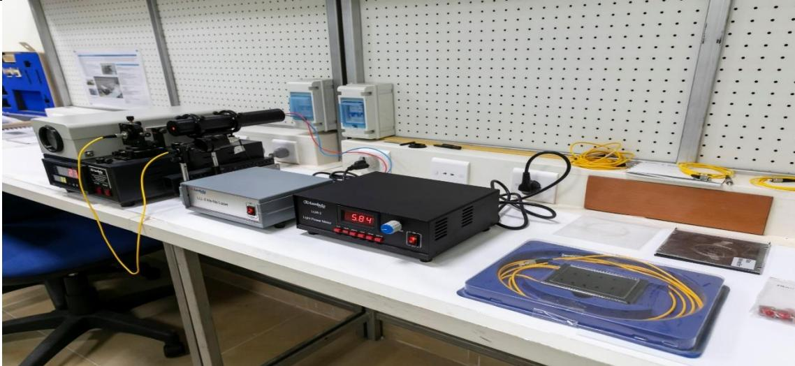
The optical fiber kit is used to understand the fundamentals of fiber optics, optical fiber coupling and the main losses parameters in the fiber. We can measure the numerical aperture of a multimode fiber, optical fiber transmission loss and Mach Zehnder optical fiber interference. In addition, the device is a temperature and pressure sensitive and use optical splitters.
